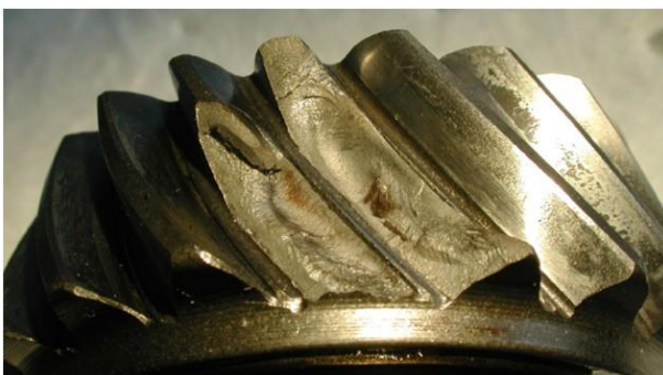
Fig. 4: Typical tooth root breakage ( a = 0 \text{ mm} )
